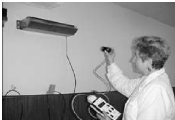
Fig. 3.7. Measuring the effectiveness of UVC 254 and the safety of fixtures at eye level using a radiometer
