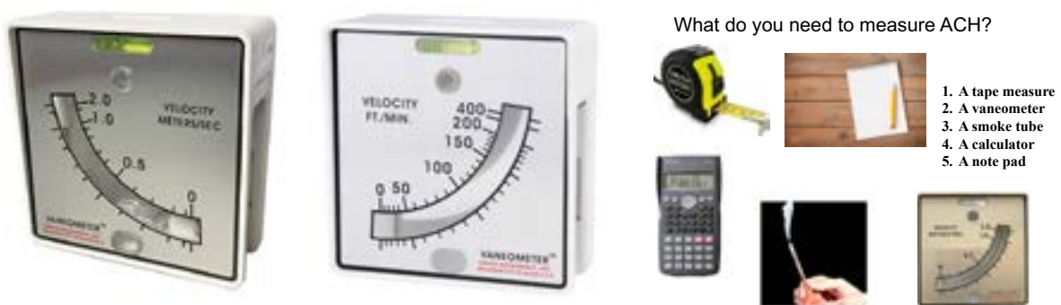
Fig. 3.11. Tools to measure ACH (including example of vaneometer with different units)
