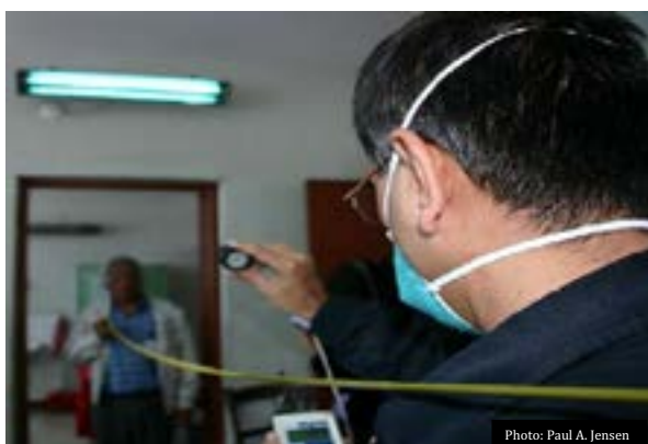
Fig. 3.7. Measuring the effectiveness of UVC 254 and the safety of fixtures at eye level using a radiometer
